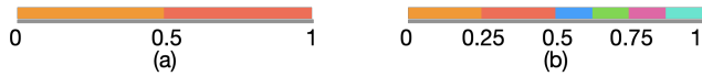
Figure 3: (a) An job-fair statistical token assignment example with two jobs. (b) A user-then-job-fair statistical token assignment of a two-tier token design with two users, one running two jobs and the other running four jobs.
