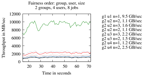
Figure 9: Four competing jobs, two from each user. Total throughput is balanced between users and between jobs belonging to each user.
